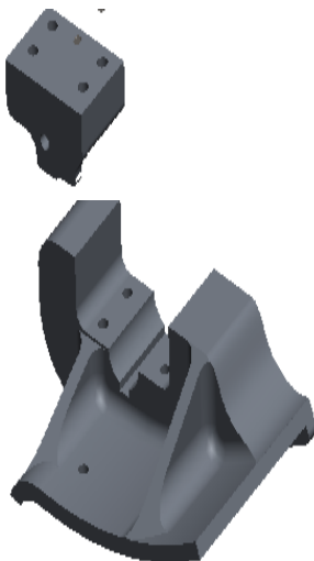
Figure 7: Leg mounts which were machined from Aluminum 6061.
