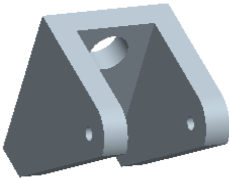
Figure 13: The mounting bracket used to affix the linear actuator to the excavation linkage.
